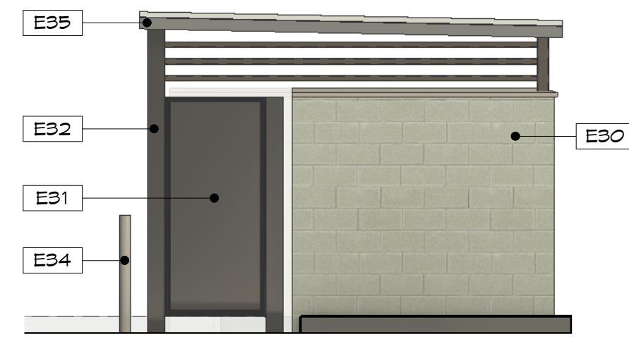
2 TRASH ENCLOSURE - EAST GSR ELEVATION 1/4" = 1'-0"
